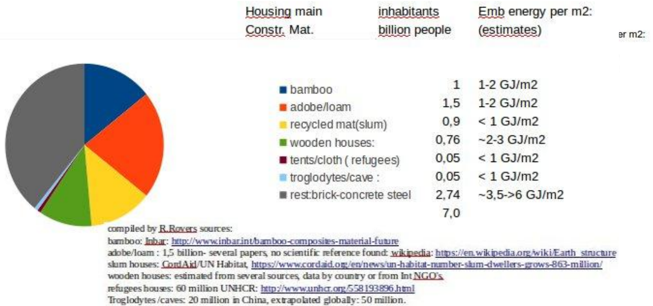
Figure 3: Living condition of human population in the built environment. Share of the different type of construction and their associated embodied energy.
